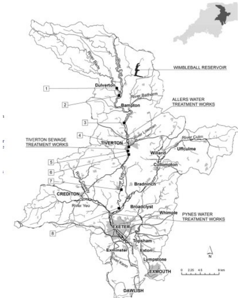
Figure 10: River Exe catchment showing the eight locations for the Chemcatcher® deployments
