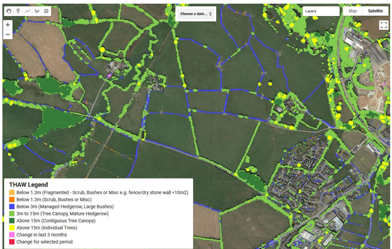
Fig 1: Screenshot from the Tree Hedgerow and Woodland (THaW) mapping and change detection tool showing an example from a mixed agricultural/urban extent in North Devon, UK. The coloured pixels correspond to the classes of tree and woodland defined in the legend. Small areas of woodland, mature and managed hedgerow, and individual/emergent mature trees, can all be seen within this relatively small extent.
