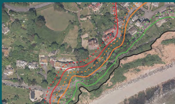
Current cliff position (black line) with predicted cliff retreat and buffer zones over 20, 50 and 100 years
