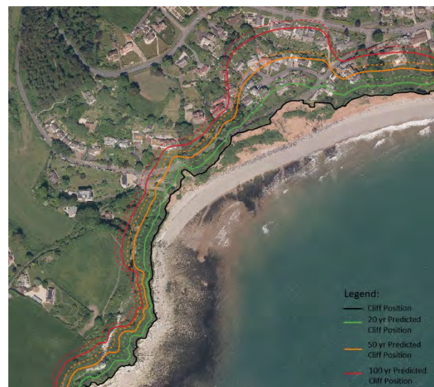
Projected future cliff position for different epochs; buffers allow uncertainty to be visualised.
